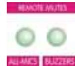
The remote mute ALL MICS switch carries out the function upon pressing it. This means that the units (belt packs, desk stations units, etc.) connected to the system can turn on the microphones again when it's required. When this switch is pressed, its associated LED turns on during a moment.
